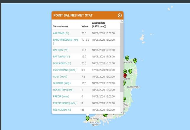
Homepage of the online hydromet data platform developed to automatically collect and process data from the 33 hydromet stations installed under the PPCR project in Grenada.
