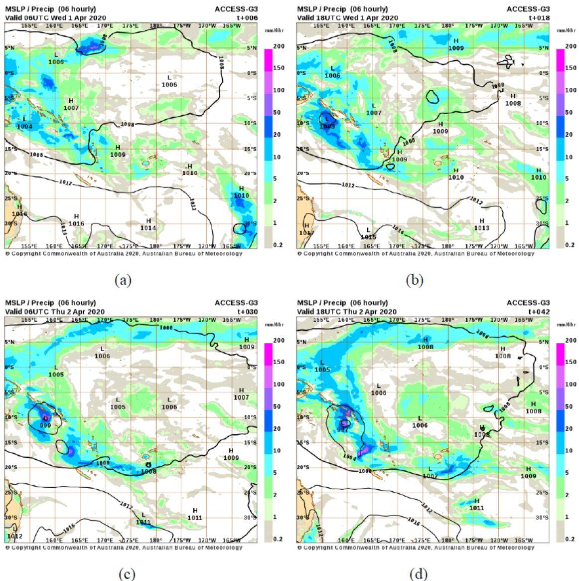
Figure 4 - Numerical model guidance for four different time steps during the formation stages of Tropical Cyclone Harold. Source: Australian Bureau of Meteorology, through SIMS TC Harold evaluation report. This shows a broad regional model view, as no Solomon Islands-specific view is available from the Bureau for these models.
