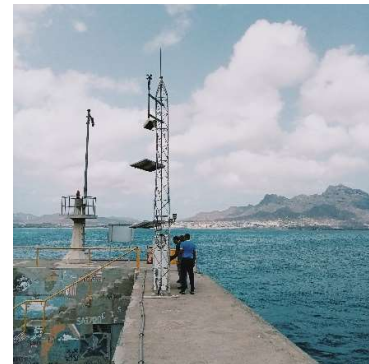
Fig. 2: Maritime AWS of Mindelo harbor on San Vicente Island; type Sutron
