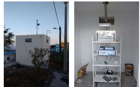
Fig. 7: Air quality monitoring in Cova Figueira, Fogo, used by INMG (near the Fogo stratovolcano)
