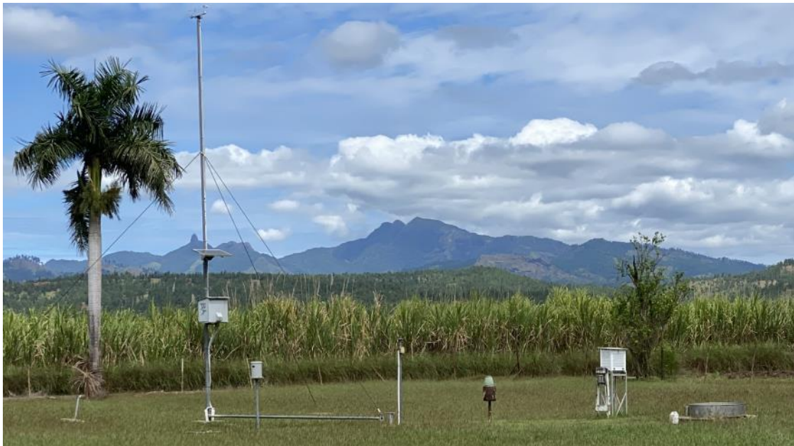
Figure 7 - An example Automatic Weather Station (AWS) and manual station setup (Rarawai Mill AWS, Ba, Viti Levu), recording rainfall, maximum and minimum air temperatures, wind speed and direction, solar radiation, humidity, station atmospheric pressure, and evaporation. The AWS is a typical installation by New Zealand’s NIWA, with a tilting mast so that lofted parts can be serviced at ground level. A nearby hydrological station records river levels. Photo: Authors.
